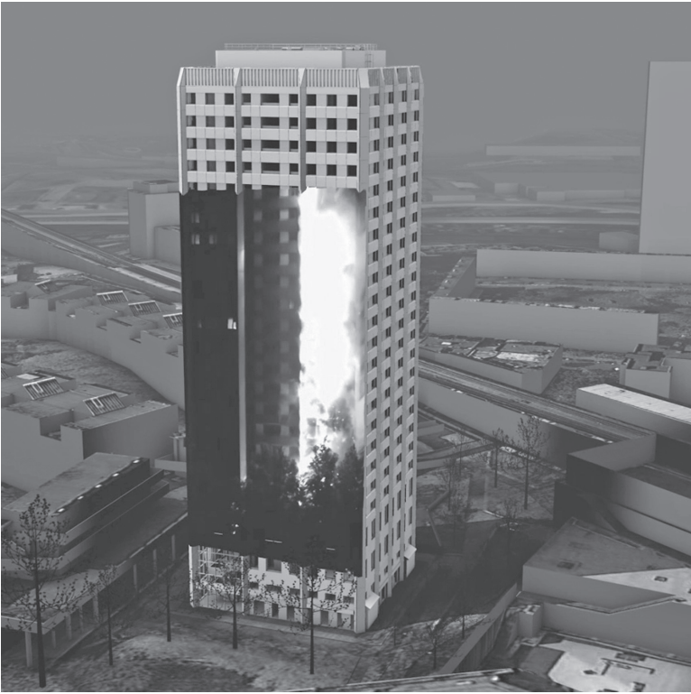
Figure 15.2 Image from Forensic Architecture, The Grenfell Tower Fire (2017–ongoing). Video footage of the 14 June 2017 fire is mapped onto a 3D architectural model of Grenfell Tower (Image: Forensic Architecture, 2018. Reproduced by permission)
